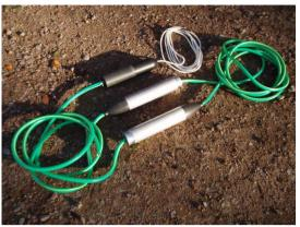
Does not meet ETSI low power GPR licensing requirement. A nonoperational licence can be applied for in the UK and Europe. Size: 390mm long, 75mm dia.
